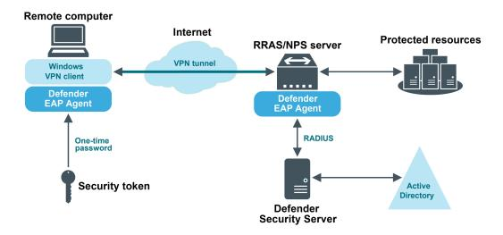
In this scenario, a component called the Defender EAP Agent must be installed both on the VPN client computer and VPN server. Extensible Authentication Protocol (EAP) is a general protocol for authentication that also supports multiple authentication methods, such as Kerberos, token cards, one-time passwords, certificates, public key authentication, and smart cards.
