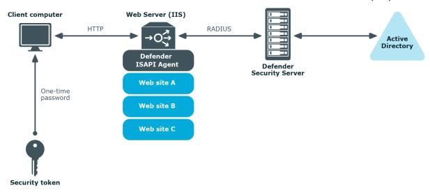
In this scenario, the Defender ISAPI Agent must be deployed on the Web Server that hosts the Web sites to be secured with Defender. The ISAPI Agent acts as an ISAPI filter and requires users to authenticate via Defender in order to get access to the Web sites hosted on the Web Server.
