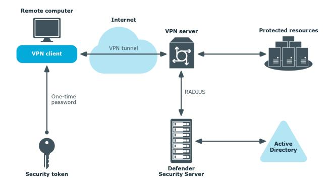
In this scenario, the VPN server is configured to redirect the user to the Defender Security Server, which prompts the user to submit a passcode. The user needs to generate a passcode by using a security token provided by Defender administrator. The Defender Security Server validates the passcode entered by the user, and if the passcode is correct allows the user to establish a VPN connection.
