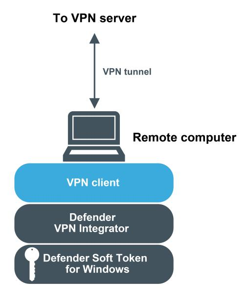
To do so, you need to install the Defender VPN Integrator on the computer where the Soft Token for Windows is installed. When the user initiates a VPN connection, VPN Integrator
