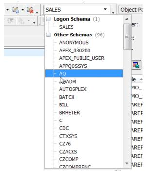
By default, the current schema is set to your current connection. When you use this drop-down, Toad issues an ALTER SESSION SET current\_schema command. After you execute, Toad issues the ALTER SESSION SET current\_schema command again to return to the original connection schema.
