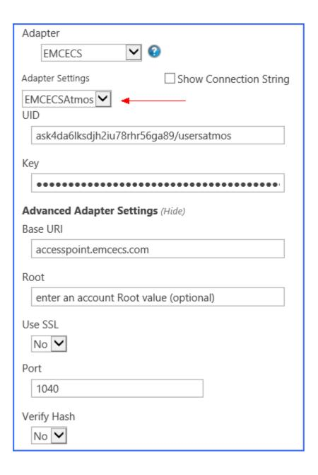
Click the *Show Connection String* checkbox to edit the connection string. Otherwise, fill in the connection fields shown for the adapter selected. Notice that the connection string parameters are name/value pairs separated by semi-colons.
