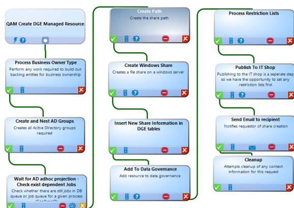
Figure 2: QAM Create DGE Managed Resource process chain
