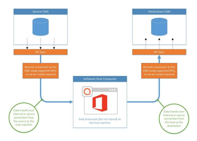
As we will discuss a little later, any obstacles or hurdles that sit in the process of this data flow (load balancers, firewalls, antivirus scanners, VPN, etc.) may have a negative impact on throughput. Wherever and whenever possible, we want to establish a path of least resistance.
