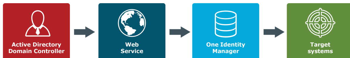
Figure 1: How the password synchronization feature works
