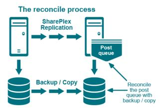
Although the **reconcile** command is designed for use in high-volume environments, it can be used in low-volume environments with an understanding that the reconcile process can, in some circumstances, seem to stall. This happens because the **reconcile** command depends on data continuing to arrive from the source system. If there is no replication activity on the source system after the hot backup or copy, the reconcile process waits until source activity resumes.
