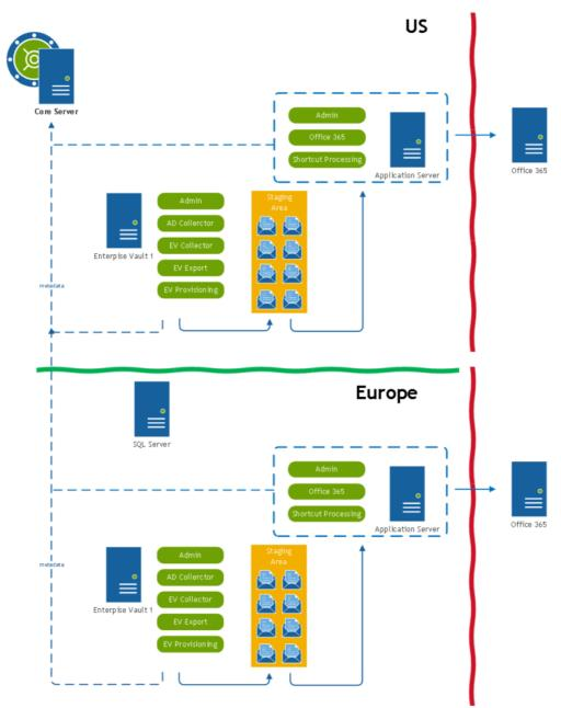
In this situation, one Core can still be deployed. The modules will receive commands and transmit metadata over the corporate network. The export/import is done within each geography.
