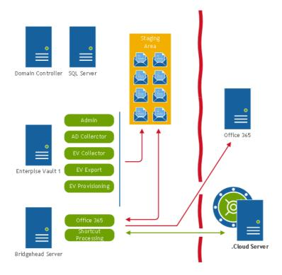
If you cannot install the modules directly onto the Enterprise Vault servers, then you can install all modules on the bridgehead server or a separate bridgehead server exclusively used for the extraction of data.
