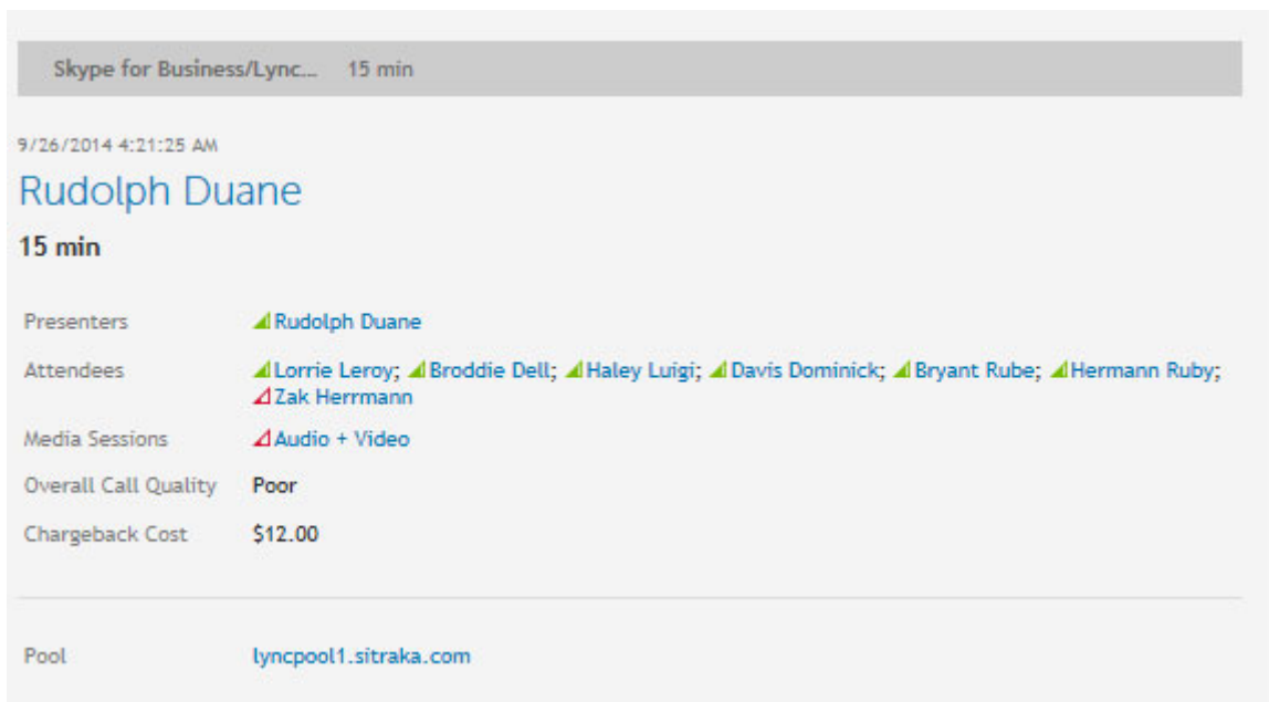
Figure 4. In the details browser, colored icons identify the individual participants that experienced good call quality or poor call quality.
