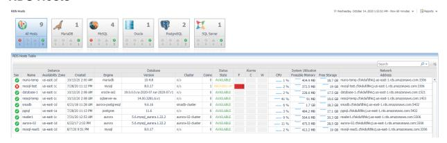
The RDS Hosts dashboard shows all monitored RDS hosts grouped by database type. Displayed for each Host are instance identity and location properties, database engine and version, current status and health, system utilization, network configuration, and Aurora cluster, if applicable. Clicking on the instance name will drill down to the RDS Host Overview page for the selected instance, while clicking or hovering on many other column values will expose more data.
