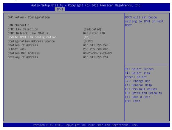
5. Stay on the **BMC Network Configuration** page, select **Configuration Address Source**, press **Enter**, and select **Static**.
