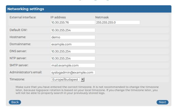
a. **External interface** — **IP address**: IP address of the external interface of SSB (for example, 192.168.1.1). The IP address can be chosen from the range of the corresponding physical subnet. Clients will connect the external interface, therefore it must be accessible to them.
