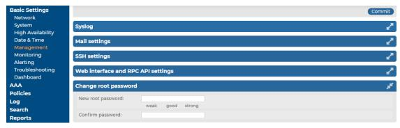
Enter the new password into the New root password and Confirm password fields. The password must meet the requirements of the AAA > Settings > Password settings > Minimal password strength option.
