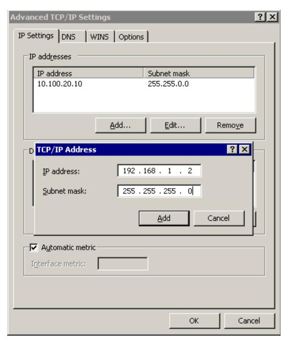
6. Into the **IP Address** field, enter **192.168.1.2**. Into the **Netmask** field, enter **255.255.255.0**.
