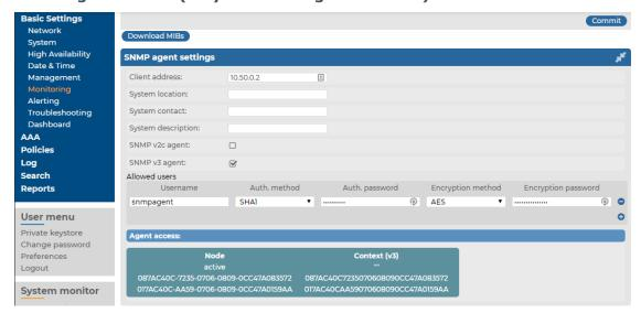
Figure 48: Basic Settings > Monitoring > SNMP agent settings — Configure SNMP agent access (both SNMP v2c and SNMP v3 agent enabled)
