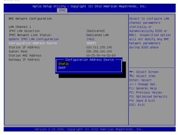
6. Still on the **BMC Network Configuration** page, configure the **Station IP Address**, **Subnet Mask**, and **Gateway IP Address** individually.
