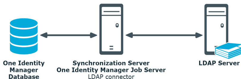
Figure 1: Architecture for synchronization
