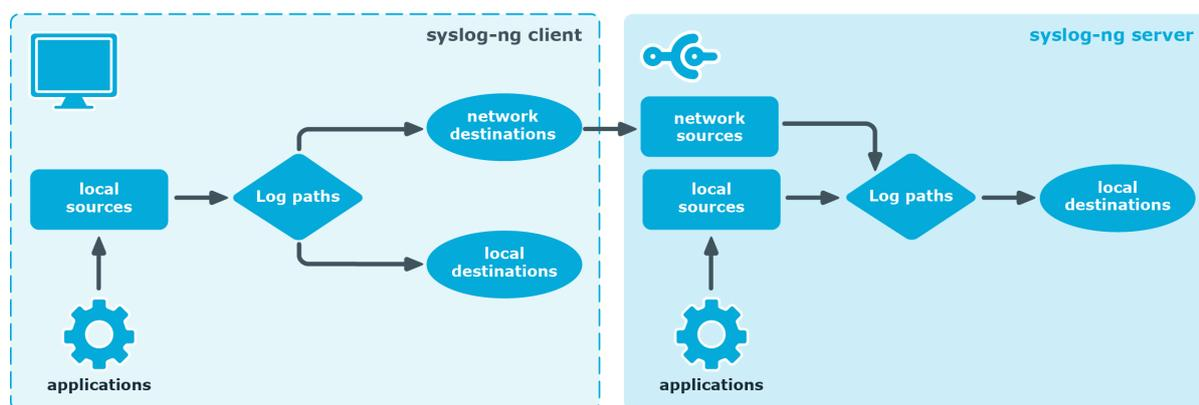
In client mode, syslog-ng collects the local logs generated by the host and forwards them through a network connection to the central syslog-ng server or to a relay. Clients often also log the messages locally into files.
