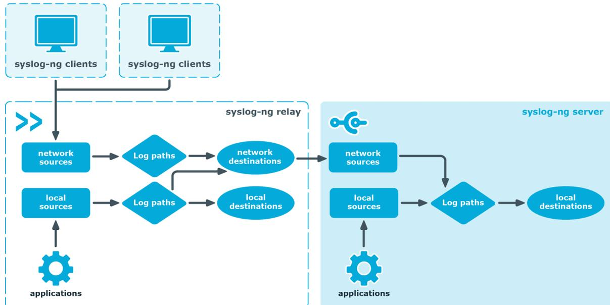
In relay mode, syslog-ng receives logs through the network from syslog-ng clients and forwards them to the central syslog-ng server using a network connection. Relays also log the messages from the relay host into a local file, or forward these messages to the central syslog-ng server.
