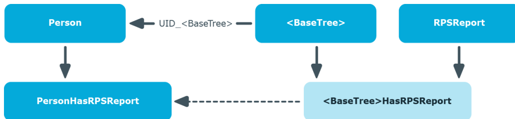
Figure 3: Inheritance with Indirect Primary Assignment of Applications to Employees
