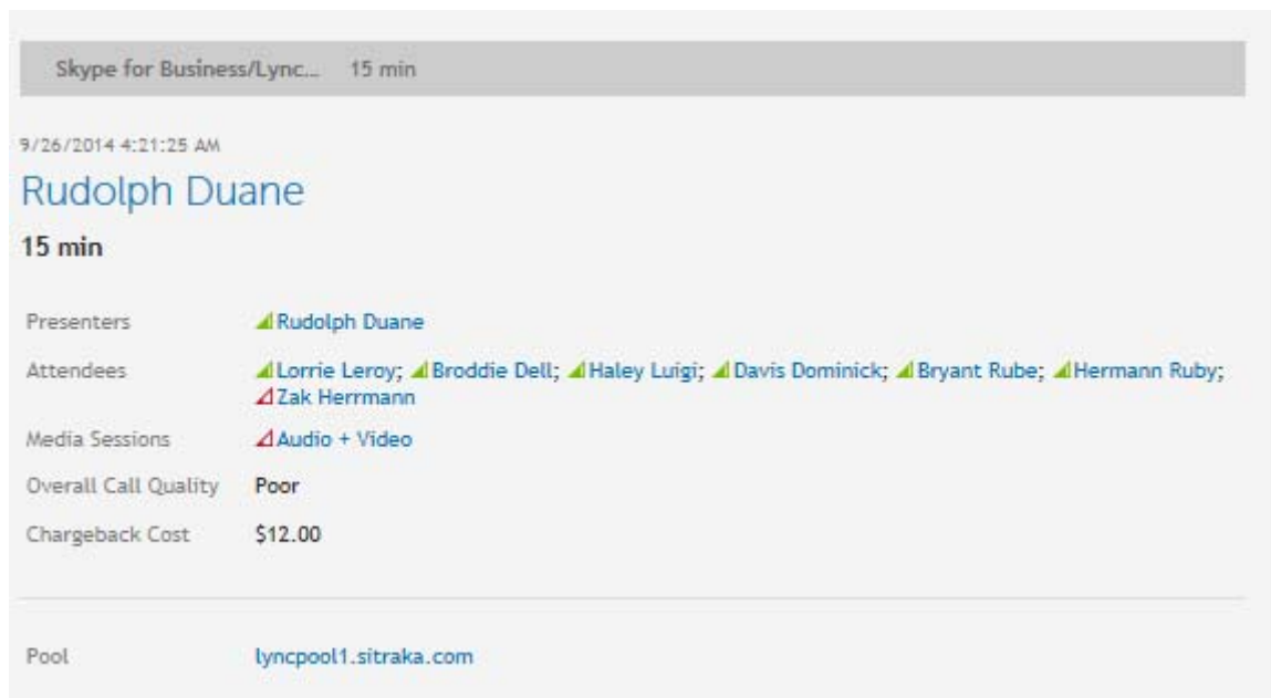
Figure 3. In the details browser, colored icons identify the individual participants that experienced good call quality or poor call quality.
