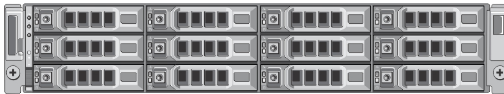
Figure 2. DR Series System Expansion Shelf (MD1200) Drive Slot Locations
