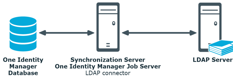
Figure 1: Architecture for synchronization
