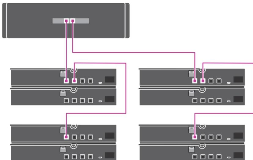
Multichain configuration supports up to four enclosures. The first two enclosures are daisy-chained with one of the enclosures connected to a single port on the controller card. The other two enclosures are daisy-chained with one of the enclosures connected to the second port on the controller card.
