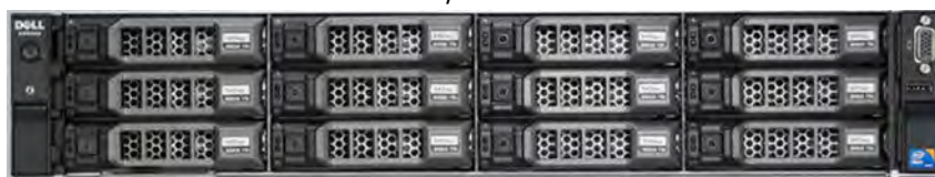
Figure 1. DR Series System Drive Slot Locations
