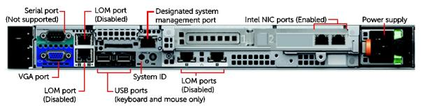
The back panel includes the following components and connectors:
